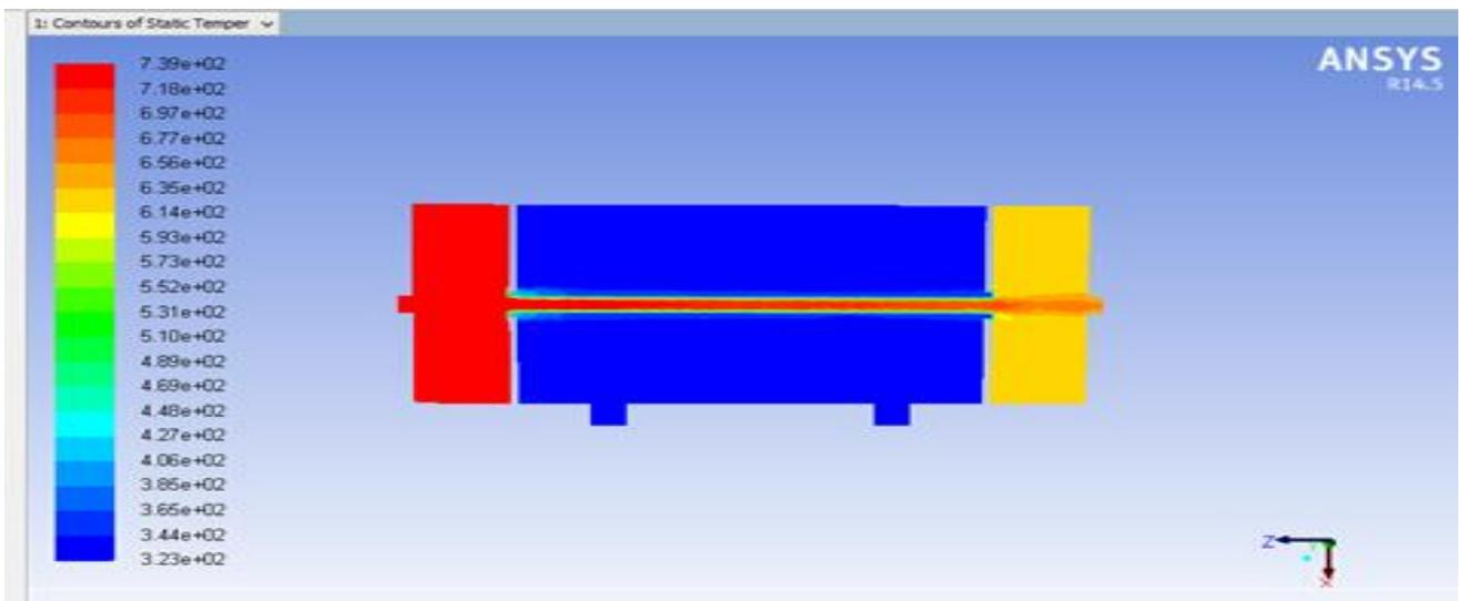
Fig. 6 temperature contour of rectangular fin tube EGR cooler
