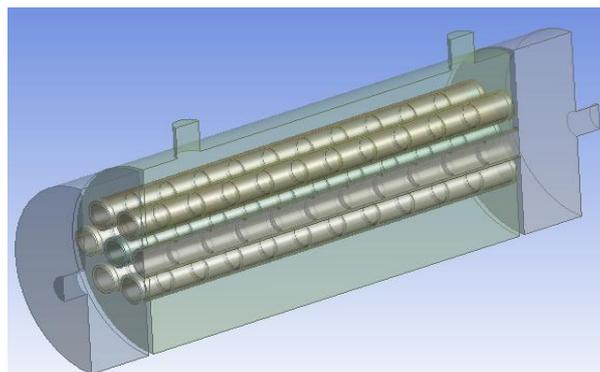
*Fig.2 Fluid model assembly of circular fin tube EGR cooler*
