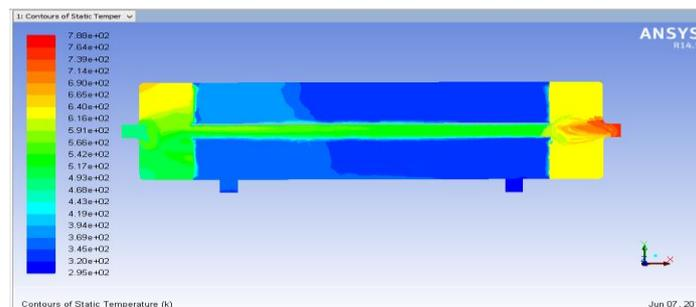
Fig. 4 temperature contour of plain tube EGR cooler
