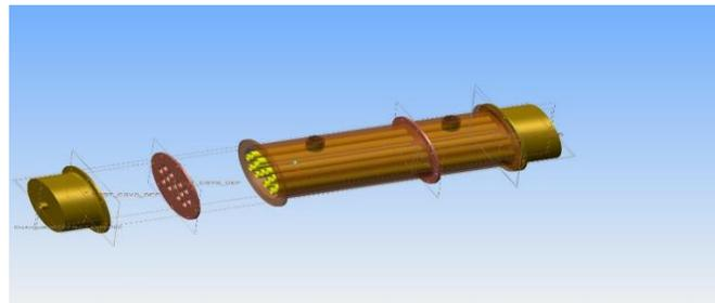
*Fig.1 Assembly of EGR cooler*
