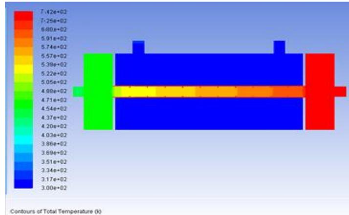
Fig. 5 temperature contour of circular fin tube EGR cooler
