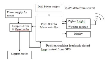
Fig 6. Block diagram of the project
