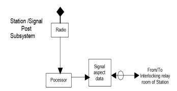
Fig 3. Station and Signal post subsystem of GPS based cab signalling
