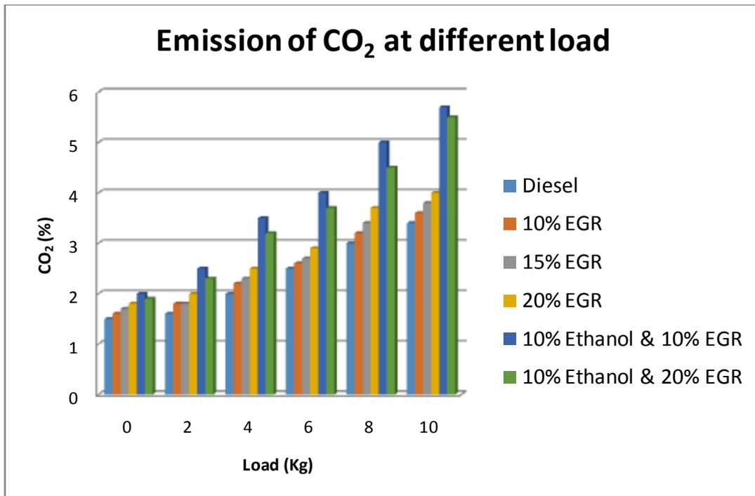
**Fig. 4** Comparison of CO<sub>2</sub> value in control and experimental groups at different load
