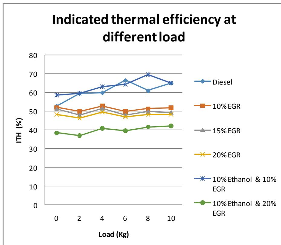
**Fig. 8** Comparison of indicated thermal efficiency at different load
