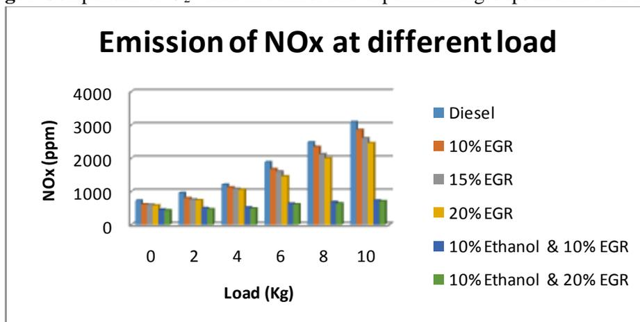
**Fig. 6** Comparison of NOx value in control and experimental groups at different load
