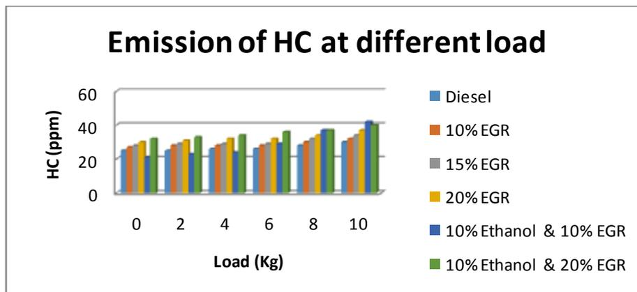
Fig. 3 Comparison of HC value in control and experimental groups at different load
