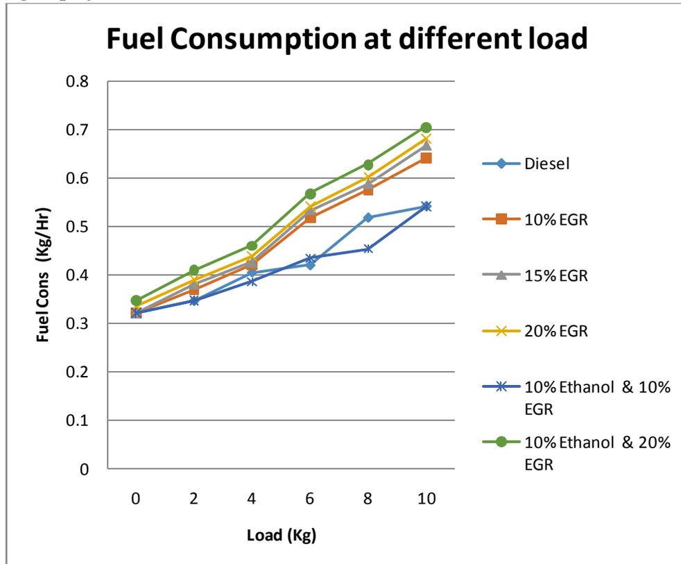
**Fig. 7** Comparison of Fuel Consumption value in control and experimental groups at different load
