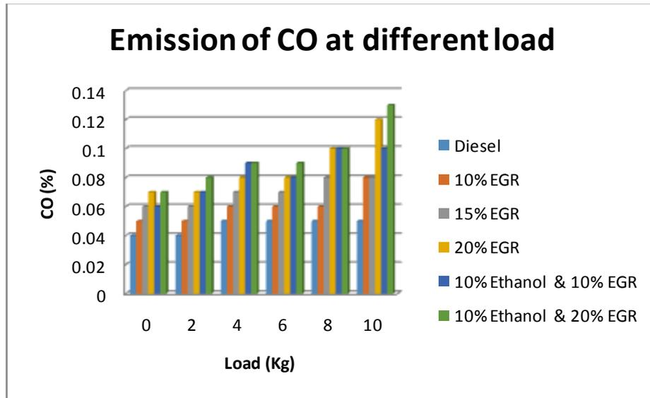
Fig. 2 Comparison of CO value in control and experimental groups at different load
