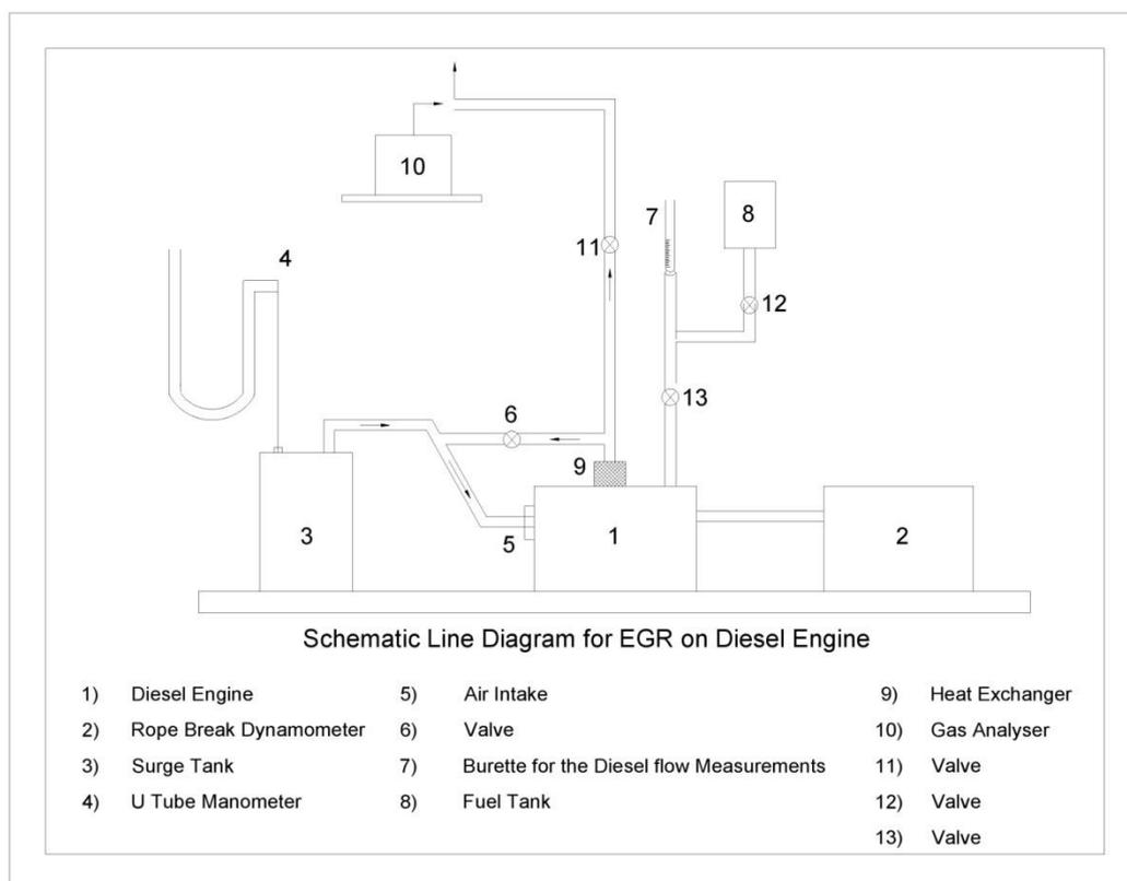
*Fig 1. Engine setup used for the experiment*
