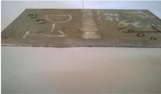
**8011 alloy welded by tapered threaded tool**
