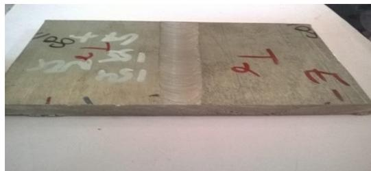
**8011 alloy welded by tapered tool**
