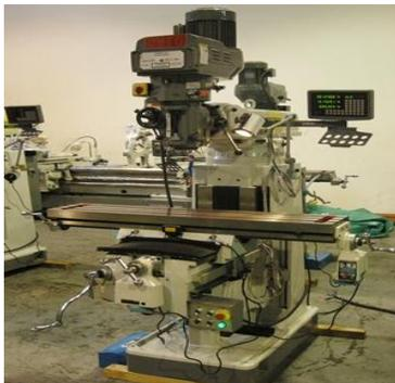
Figure 3 Vertical Milling head machine
