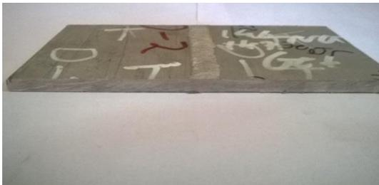
**7005 alloy welded by tapered tool**
