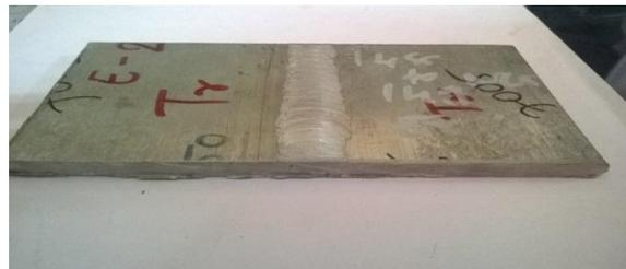
**7005 alloy welded by tapered threaded tool**
