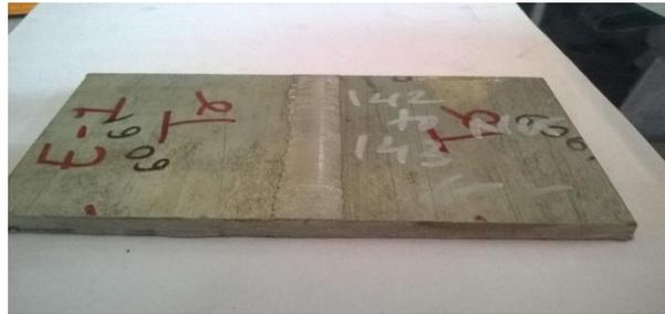
**6061 alloy welded by tapered tool**
