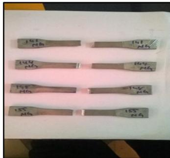
**Figure 9 Tensile test specimens after test.**
