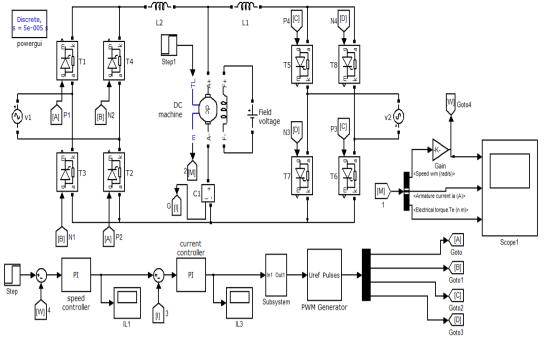
Figure 3.Closed loop Simulink model of Dual Converter
