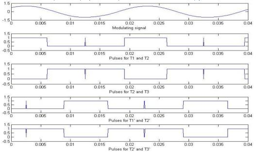
Figure 9 Modulated signal and generated pulses
