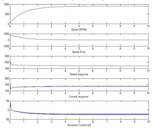
Figure 6. W\*=900 RPM at T= -7.5 N.m Speed, system response and armature current
