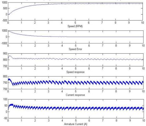
Figure 5. W\*=900 RPM at T=7.5 N.m Speed, system response and armature current
