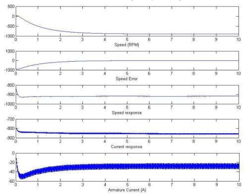
Figure 8. W\*=-900 RPM at T=-7.5n.m condition Speed, system response and armature current
