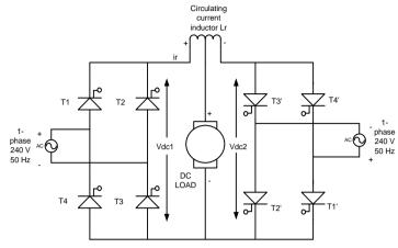
Figure 1. single phase dual converter with circulating current mode
