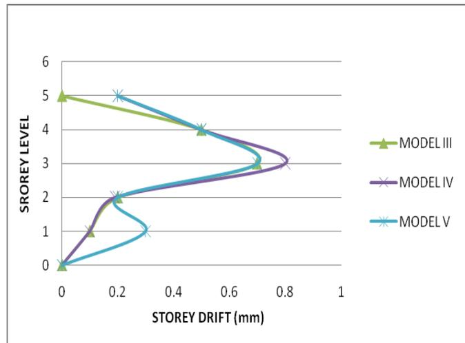
Figure 12: Comparison of storey drift in longitudinal direction
