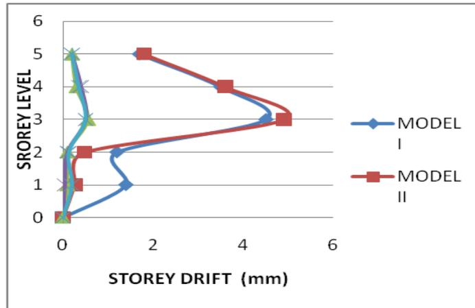
Figure 13: Comparison of storey drift in transverse direction
