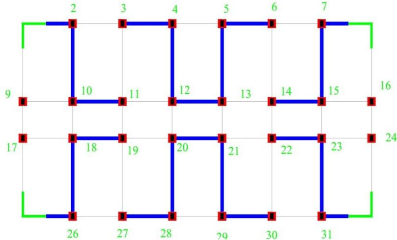
Figure 5: Plan of building with the location of infill and shear wall at parking
