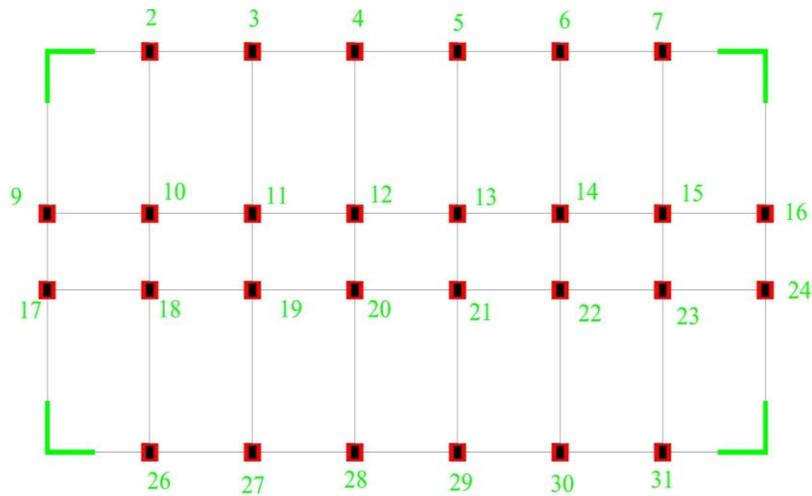
Figure 6: Plan of building with the location of shear wall at parking
