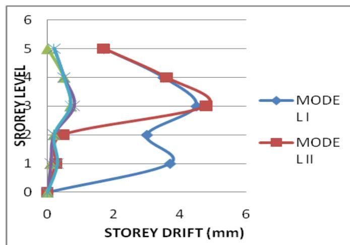
Figure 11: Comparison of storey drift in longitudinal direction
