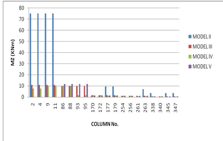
Figure 15: comparison of maximum bending moment (Mz)
