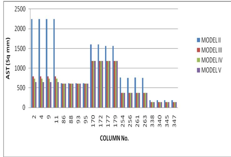
Figure 17: Comparison of steel for columns of different floors
