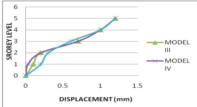
Figure 10: Comparison of displacement in transverse direction
