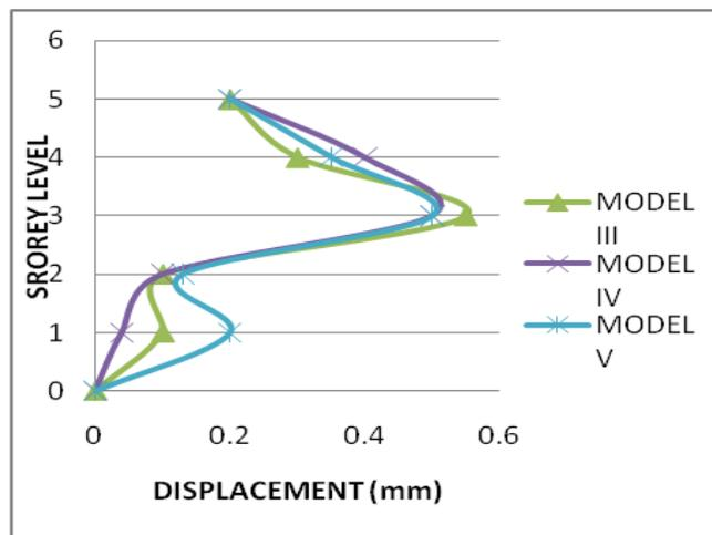
Figure 14: Comparison of storey drift in transverse direction
