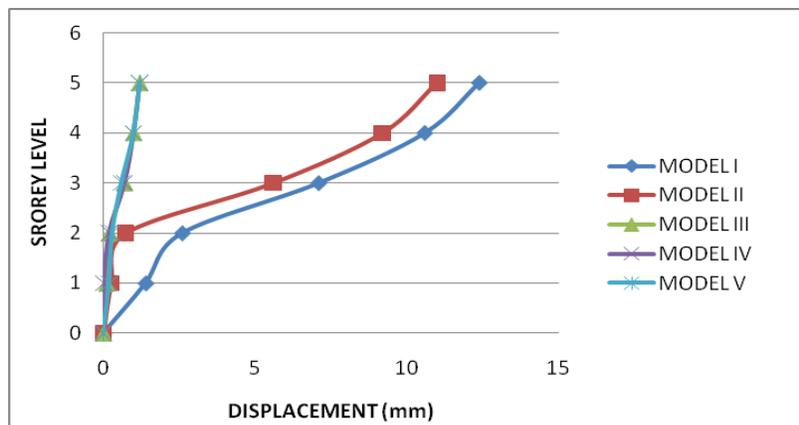
Figure 9: Comparison of displacement in transverse direction
