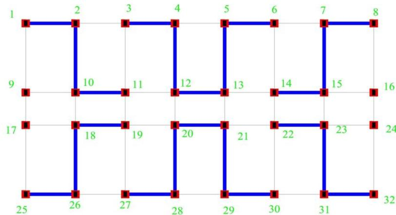
Figure 4: Plan of building with the location of infill walls at ground storey
