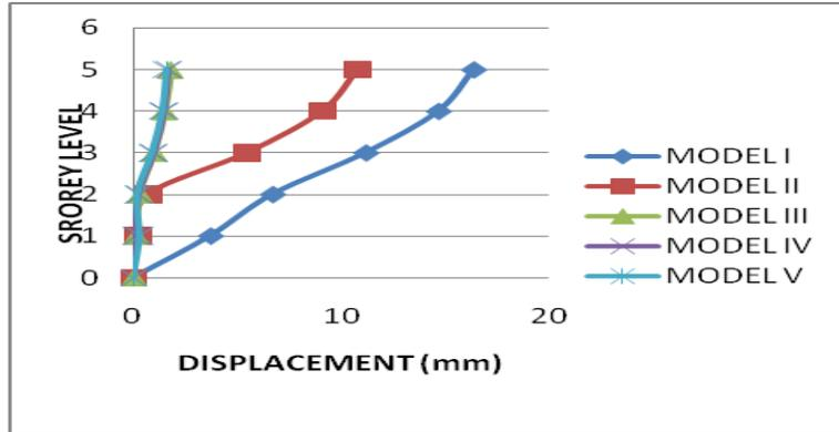
Figure 7: Comparison of displacement in longitudinal direction
