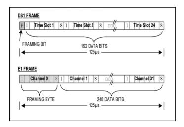
The collection of one sample from each channel is called a frame. The set of first samples of all channel is one frame, the set of second samples is called second frame and so on. The duration of each frame is 125 microseconds. Hence the frame rate is 8000 frames per second. The total bit rate of T1 line is (8000 x (24 x 8 bits) + 1 bit) = 1544000 bits per second (1.544 Mbps). This is called digital leveling signal or DS1. This was about Japanese standard and North American standard.
