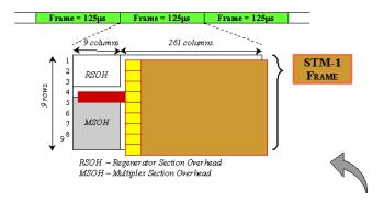
The above figure shows the frame structure of SDH. It has nine rows and 270 columns .Hence total bytes are  $(9 \times 270 = 2430 \text{ bytes})$ . Like PDH, the duration of each SDH frame is 125 microseconds. Hence the frame rate is 8000 frames per second. The left part of the frame is called Transport Overhead (TOH) which consists of three parts- Multiplier Section Overhead (MOH), Regenerative Section Overhead (ROH) and
