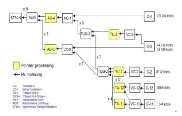
Virtual container is a container extended with a Path Overhead (POH).POH is used to control the transmission of information of the container. Tributary units TU are the units which are composed of VC11, VC12, VC2 and VC3 virtual containers along with a pointer. C11, C12 and C2 are inferior order containers. Superior order containers (C3 and C4) have the POH composed of a column of 9 bytes.
