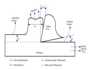
Figure.3 Clearance Angle & Rake Angle
