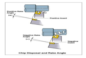
Figure.1 Rake Angle's
