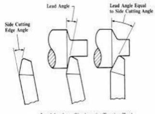
Lead Angle on Single-point Turning Tool
