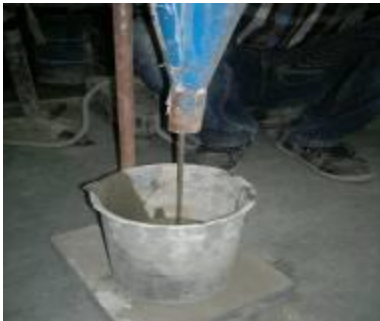
Fig: 6 Marsh Cone Test
