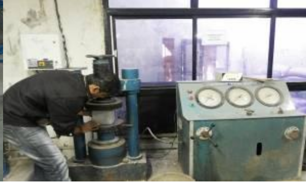
Fig: 13 Cube setting in the compression testing machine
