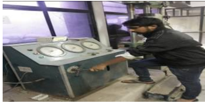
Fig: 14 Cube testing for compression
