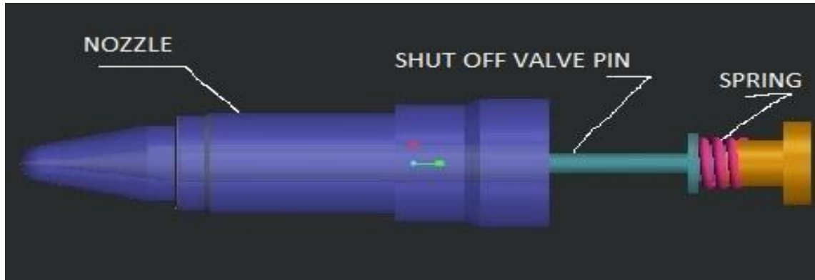
Fig 3.Secondary Nozzle with spring loaded shut off valve system:
