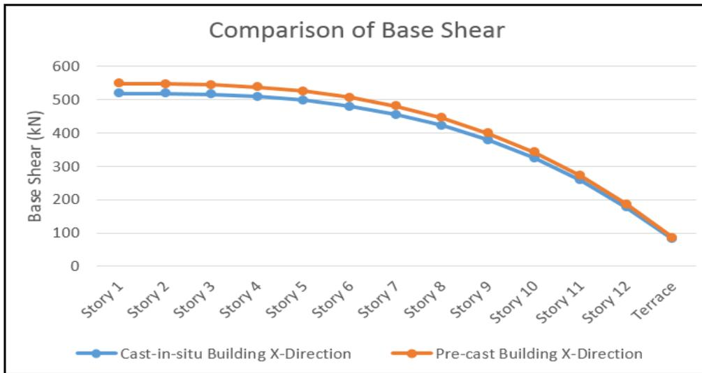
Figure 2 Comparison of Base shear in X-Direction for Both Building
