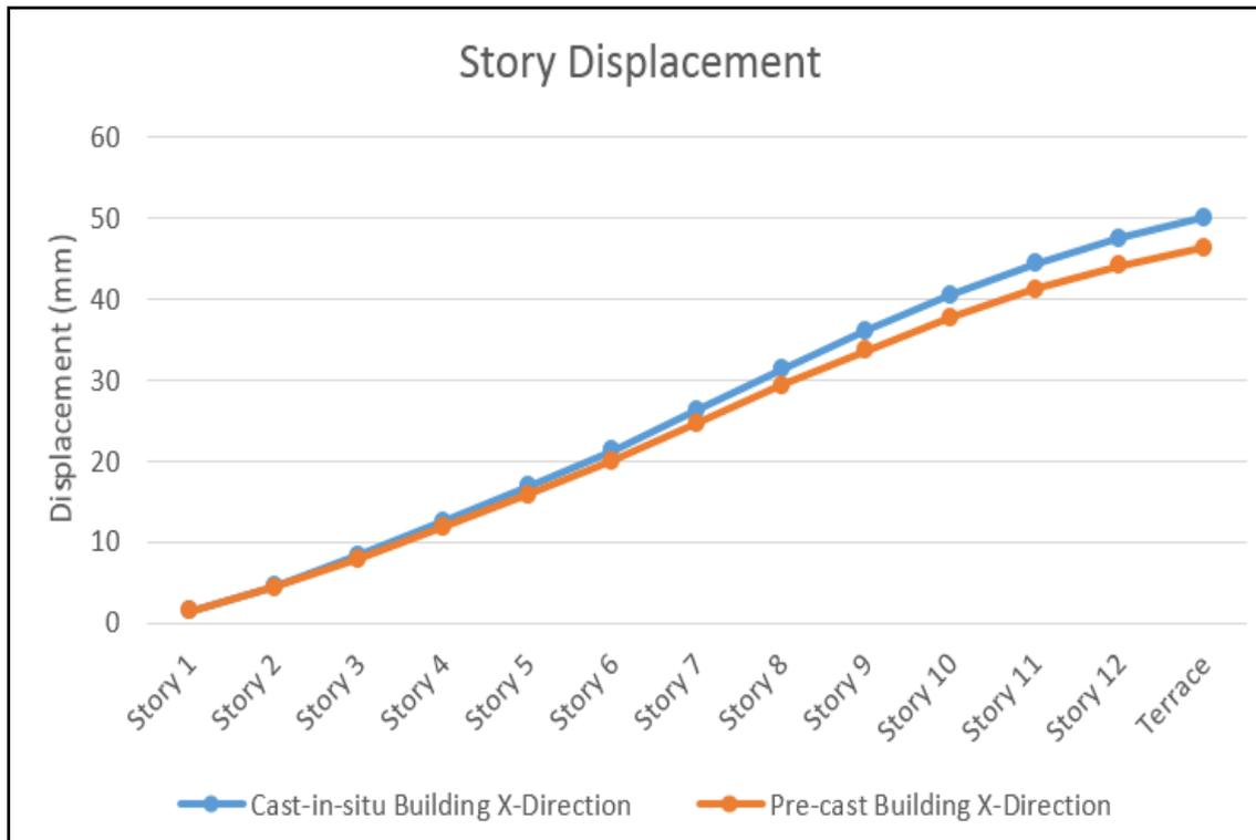
Figure 4 Story Displacement in X-Direction for both Building
