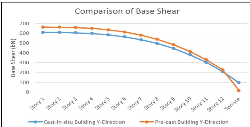
Figure 3 Comparison of Base shear in Y-Direction for Both Building
