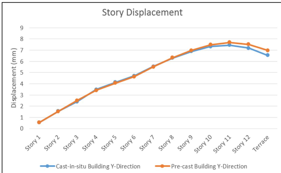
Figure 5 Story Displacement in Y-Direction for both Building
