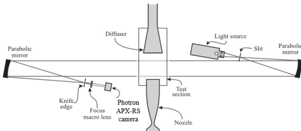
*Figure 2 Schematic setup of high-speed Schlieren photography*
