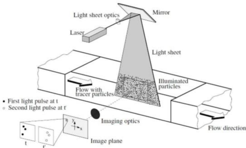
*Figure 3 Experimental Setup for PIV testing*
