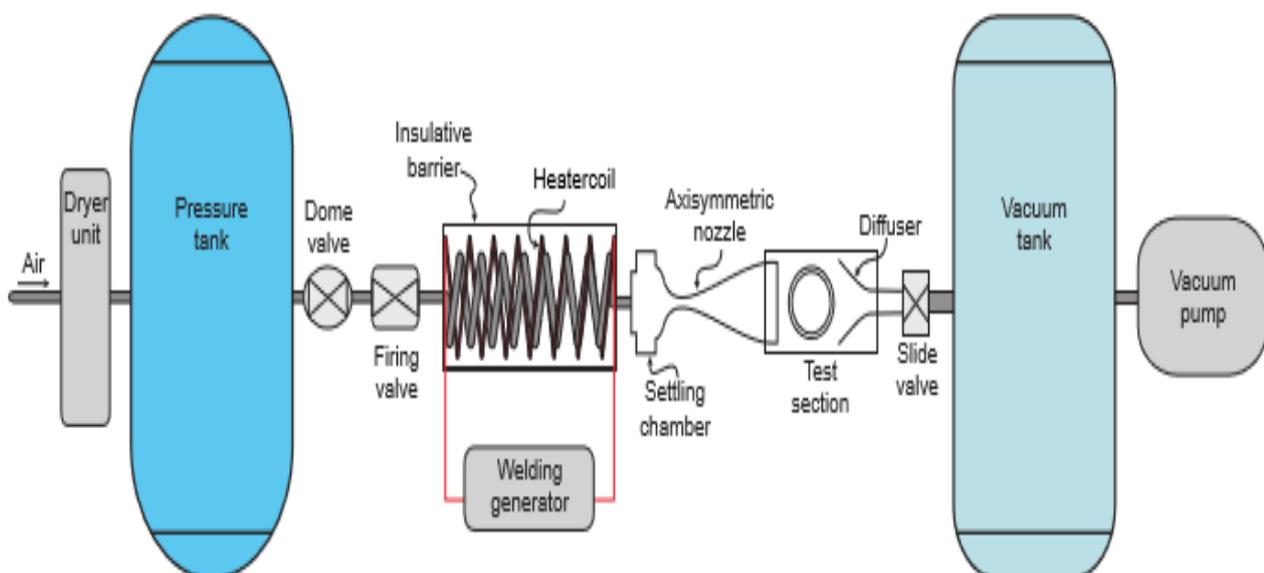
*Figure 1 Schematic layout of HSST*
