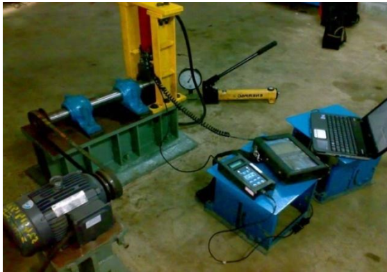
Figure 5. Test rig with AE probes
