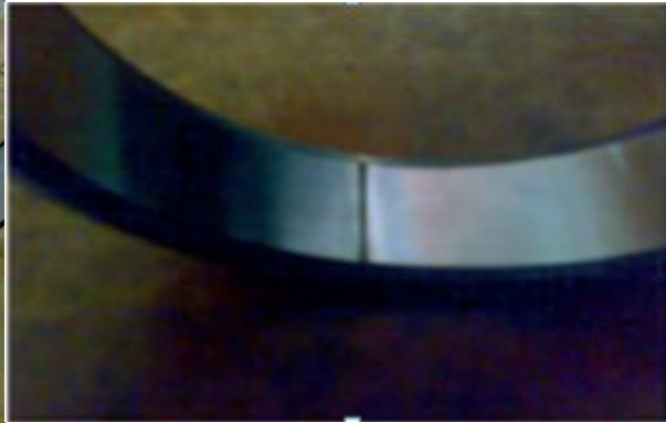
Figure 6. Outer race seeded line defect
