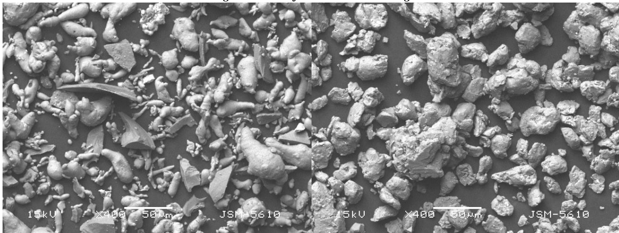
Fig 8 SEM data of hand mixing Al-SiC powder
