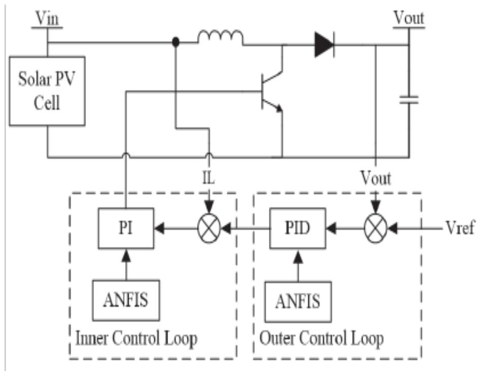
**Fig 3: Block Diagram**
