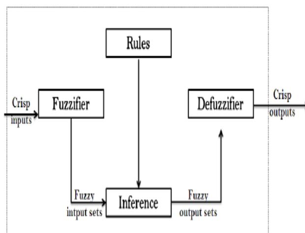
Fig.1: Block diagram of FLC
