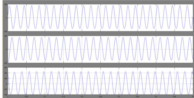
Fig 2.4 Phase voltage Four leg NPC inverter
