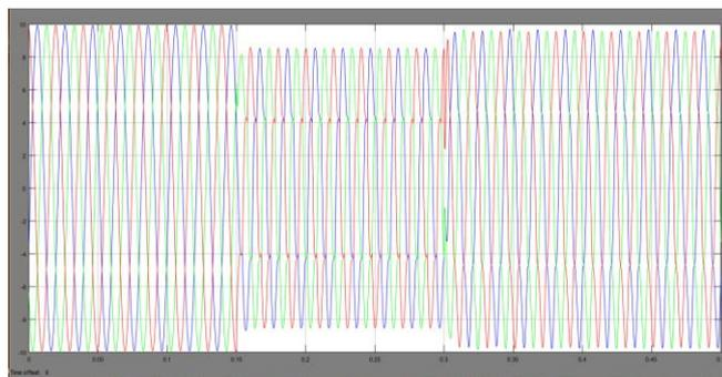
Fig 7.15 Load current Four leg NPC inverter with nonlinear load
