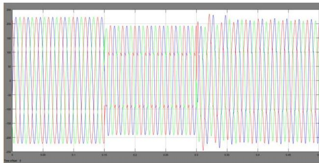
Fig 7.14 Load voltage Four leg NPC inverter with nonlinear load
