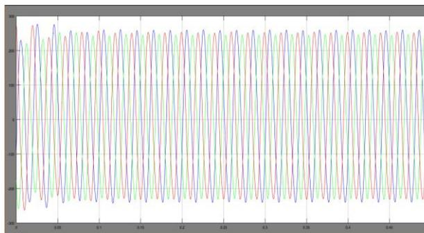
Fig 2.3 Load voltage Four leg NPC inverter
