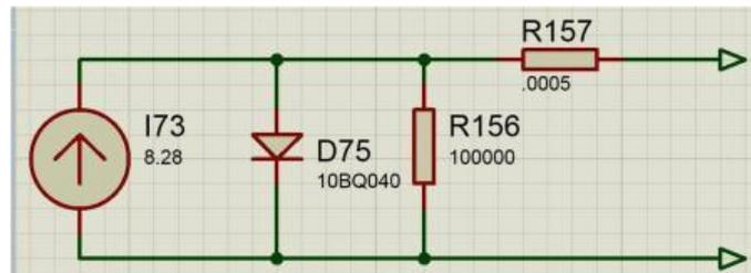
Fig.1. Single Diode Model of a Solar Cell in Proteus 8.3 Professional
