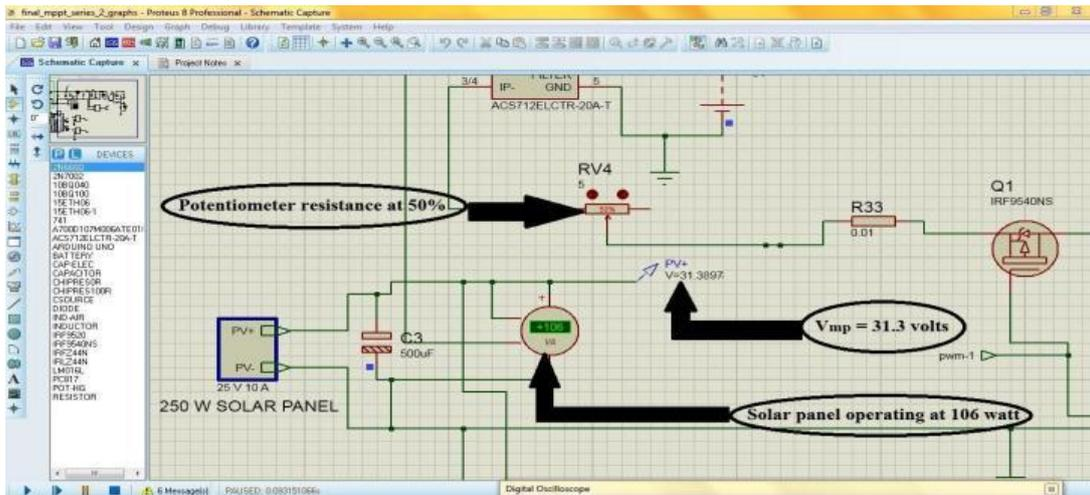
Fig.13. Potentiometer resistance at 50% & corresponding panel wattage and maximum power point voltage
