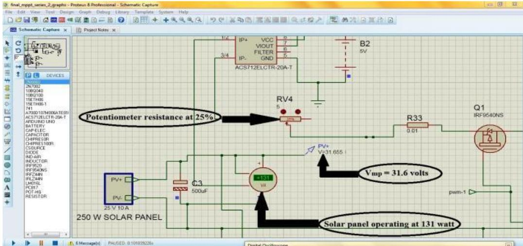
Fig.12. Potentiometer resistance at 25% & corresponding panel wattage and maximum power point voltage
