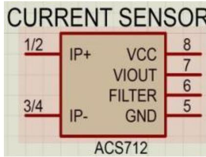
Fig.7. Current Sensor ACS712
