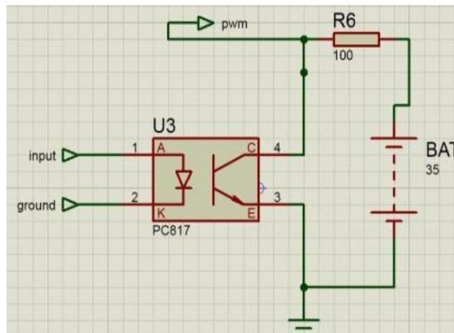
Fig.6. Gate triggering circuit consisting of PC817
