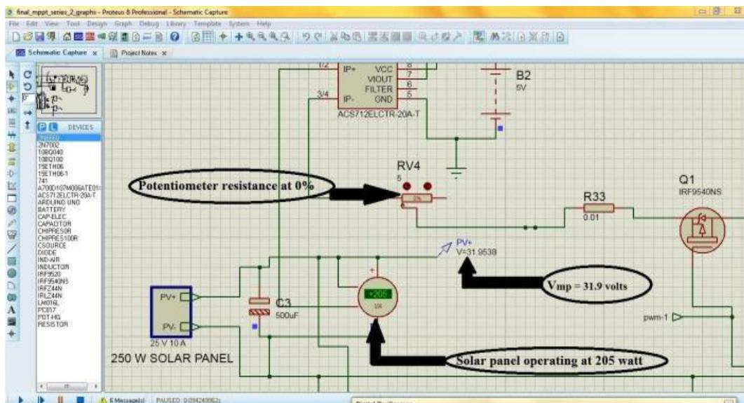
Fig.11. Potentiometer resistance at 0% & corresponding panel wattage and maximum power point voltage
