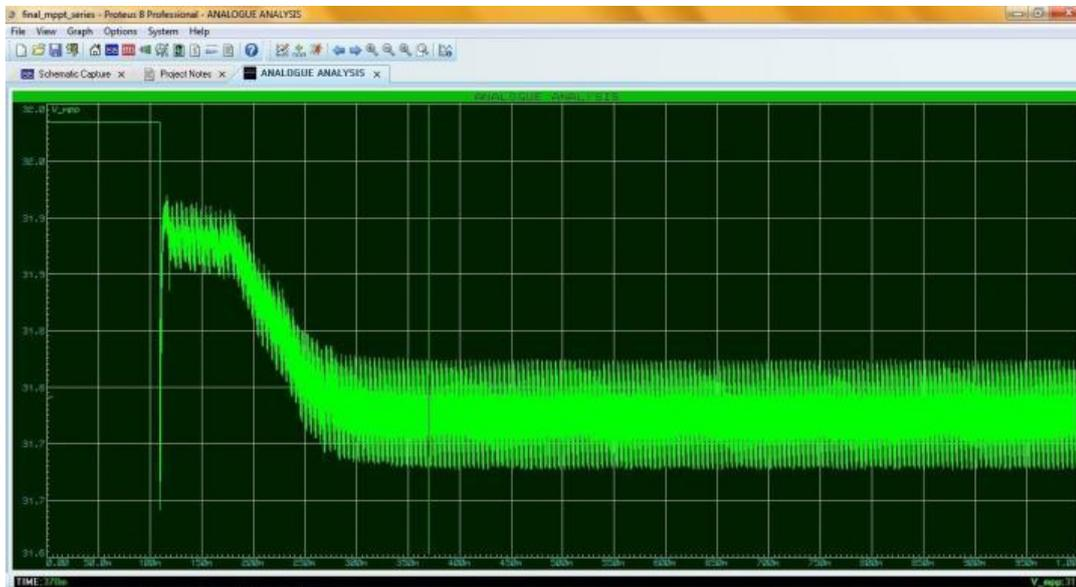
Fig. 12. Maximum Power Point voltage ( $V_{mpp}$ ) characteristics
