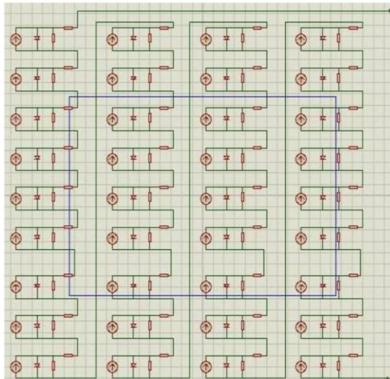
Fig.2. Configuration of 250 watt solar panel interconnecting 36 solar cells
