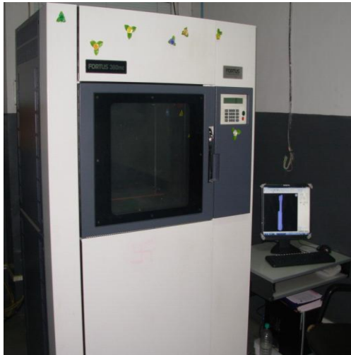
Figure3. Stratays FDM 360mc Machine setup
