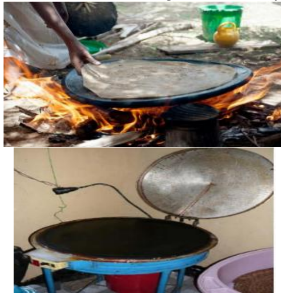
Figure. 1 a) Open fire injera baking method b) Electricity powered injera baking pan
