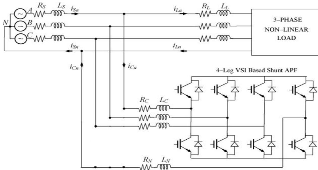
Figure.2 Four leg converter
