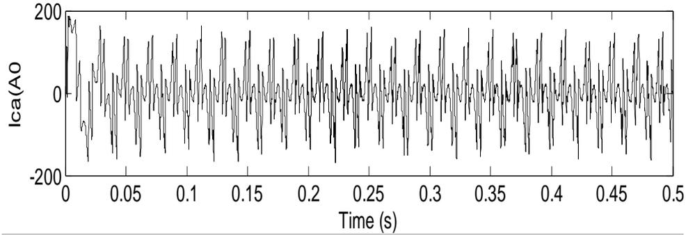
Figure 10 Compensating current waveform for phase A
