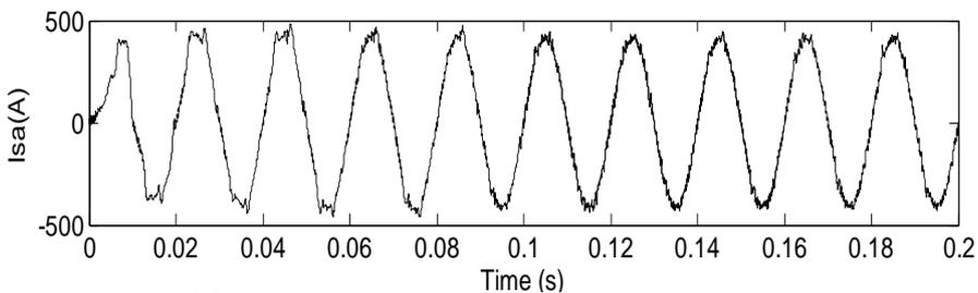
Figure 16 line current waveform for phase A with compensation
