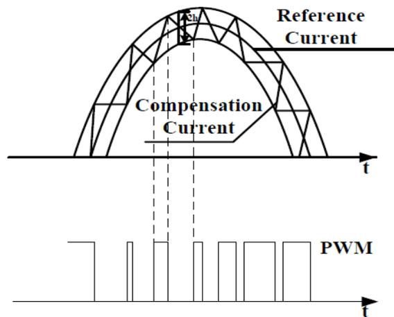
Figure 5. Current and voltage (gate) waveform with hysteresis band current control
