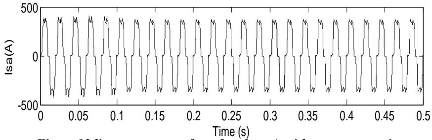
Figure 13 line current waveform for phase A without compensation
