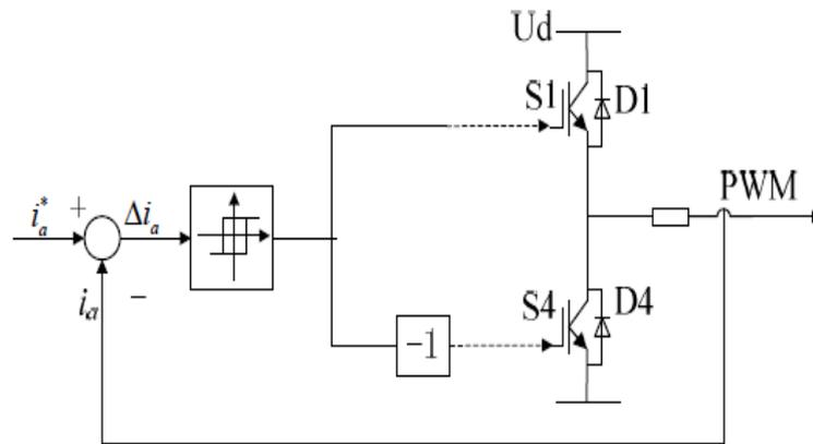
Figure 6 Circuit of current tracking control
