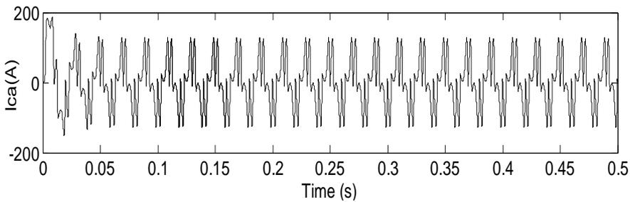
Figure 15 Compensating current waveform for phase A
