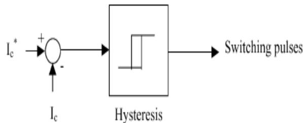
Figure 4. Conventional hysteresis band current controller.
