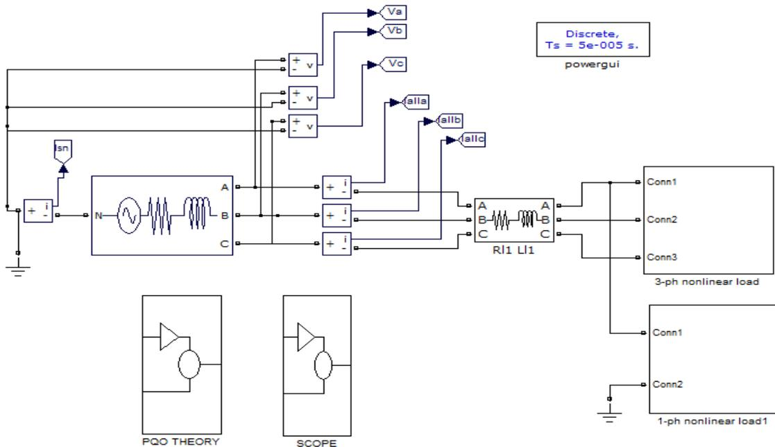
Figure 7 Matlab simulation block diagram
