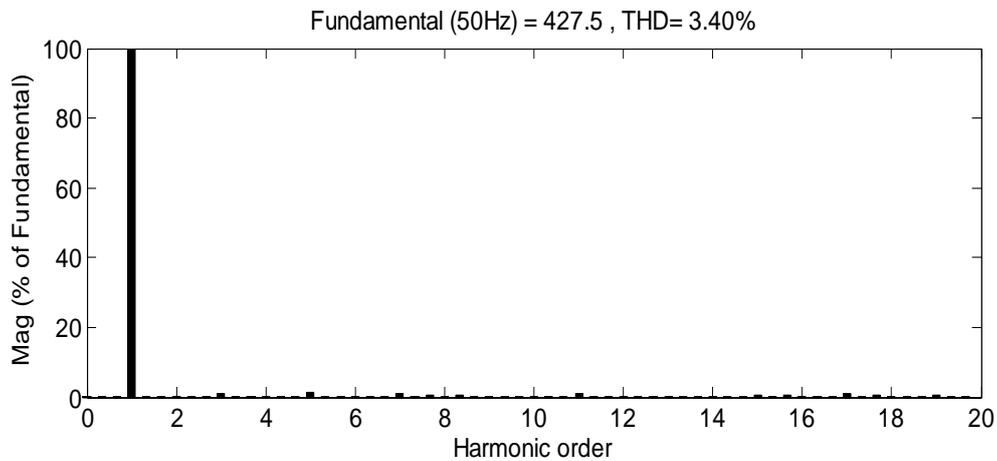
Figure 12 %THD spectrum for phase A after compensation
