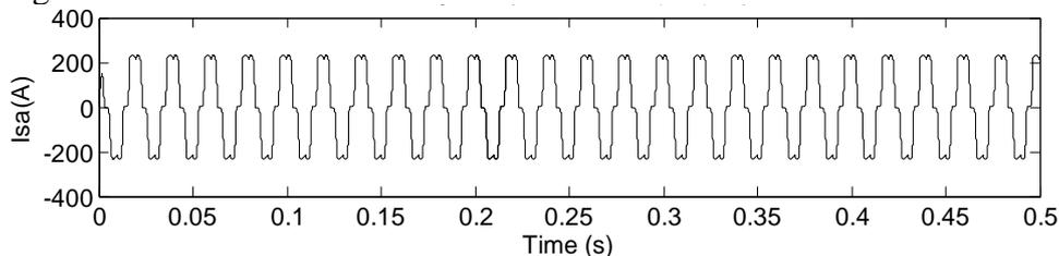
Figure 8 line current waveform for phase A without compensation
