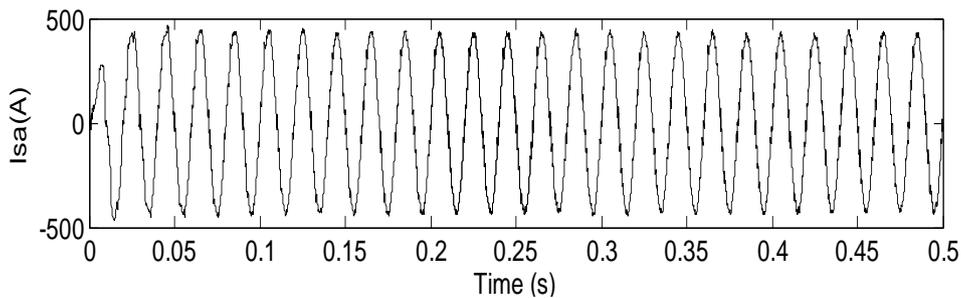
**Figure 21 line current waveform for phase A with compensation**
