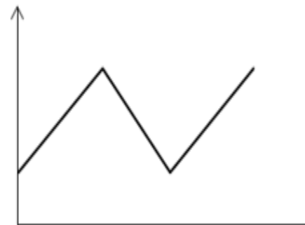
Fig 2: CCM of Buck Converter
