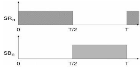
Figure 4 Switching scheme for triggering gate
