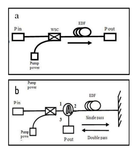
Figure 1. (a) One -stage single pass (b) one- stage double pass.
