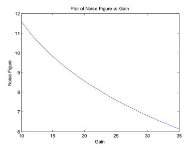
Fig.5 Gain VS Noise Figure
