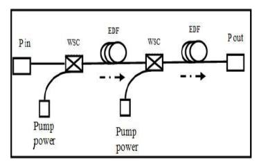
Figure 2. Two-stage double pass
