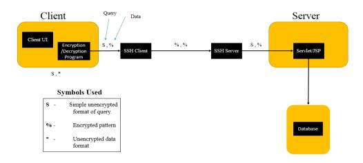
Fig-1 Architecture diagram
