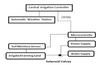
"Figure 1. Block Diagram of Automated Irrigation using ASW"
