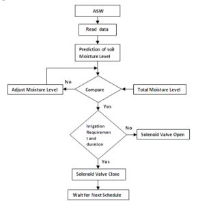
"Figure 3 . Dicision making of Irrigation Control Module"
