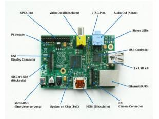
Figure 1. Raspberry Pi Model B
