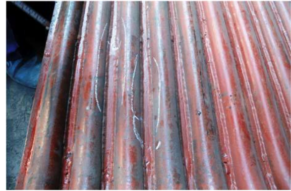
Figure 3: Shows Butt joints of fin are not ground flushed
