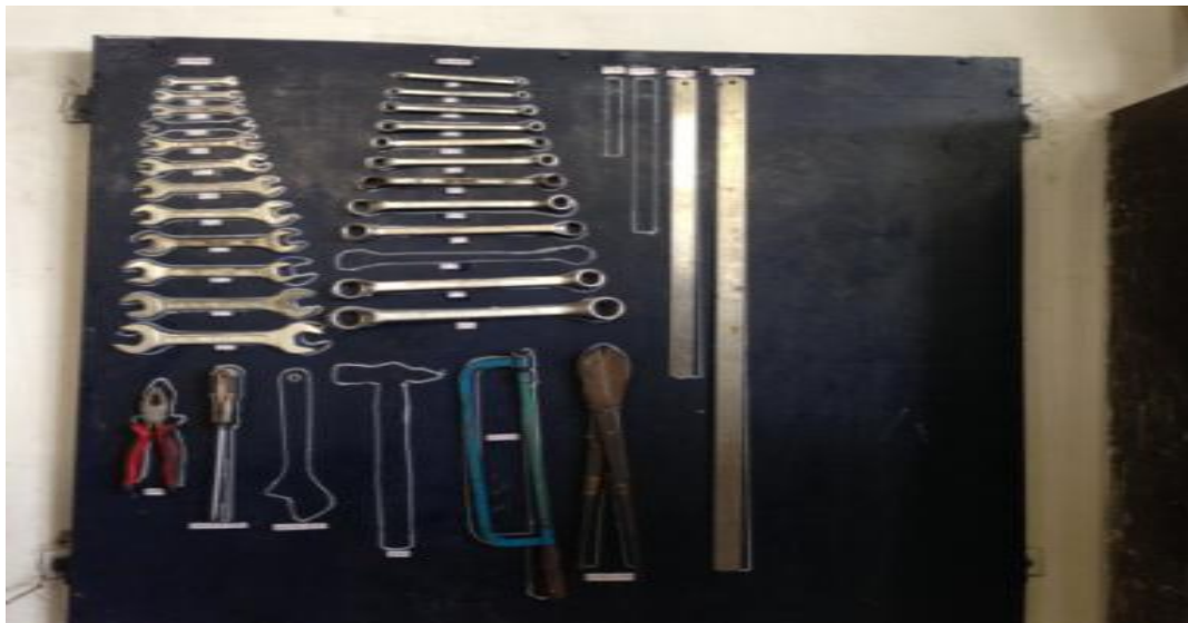
Figure 7: The "Shadows" Match the Shape and Size of the Tools
