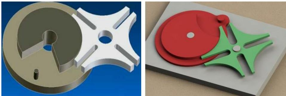
*Figure 6. Geneva Mechanism*
