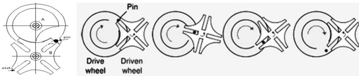
Figure 1. Indexing Mechanism
