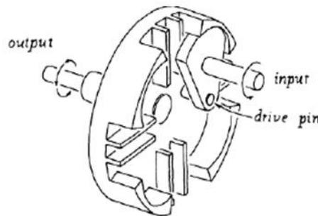
Figure 3. Internal Geneva Mechanism
