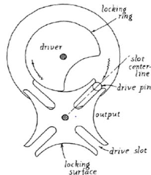
Figure 2. External Geneva Mechanism
