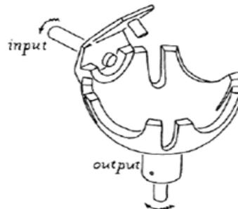
Figure 4. Spherical Geneva Mechanism
