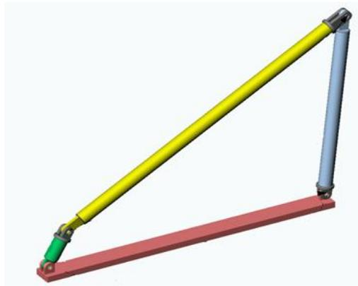
*Figure 5. Four Bar Chain Mechanism*
