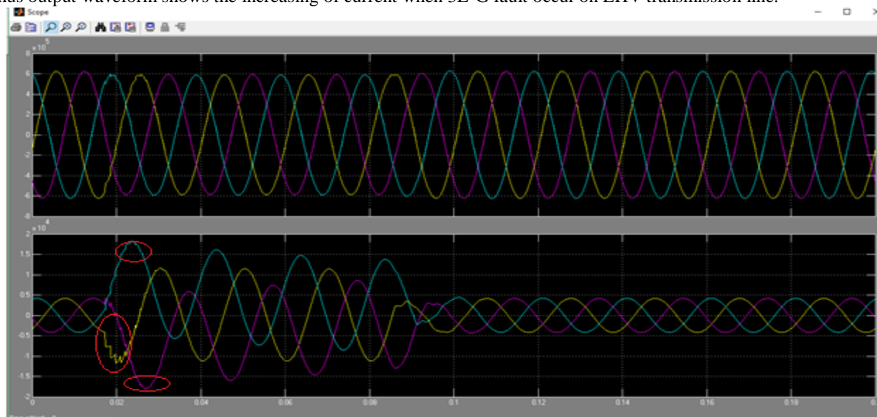
Figure: 11 LLL-G Fault waveform of current at input side in P.U.
