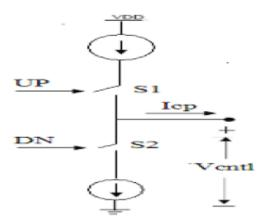
Fig. 2: Basic Block Diagram of Charge Pump
