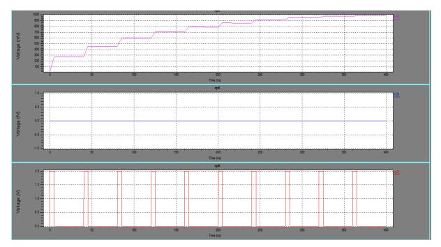
Fig. 4: Charging Waveform of the Charge Pump
