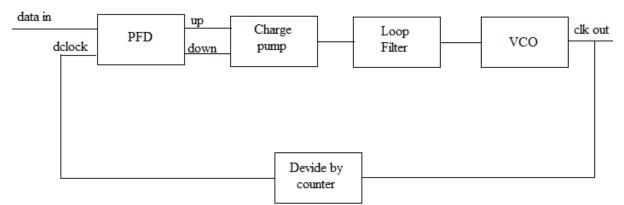
Fig. 1 A Basic Block Diagram of Phase Locked Loop
