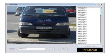
When vehicle enter into parking lot system can automatically detect the number plate (shown in fig).
