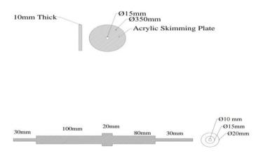
• **LIST OF COMPONENT:** 1) DC gear motor . 2) Solar panel for battery charging. 3)Battery to store and supply power to motor. 4) Oil Skimming Disk. 5) Bearing. 6)Floating tube. 7)Solar panel specification
