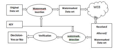
Fig1: Digital watermarking scheme
