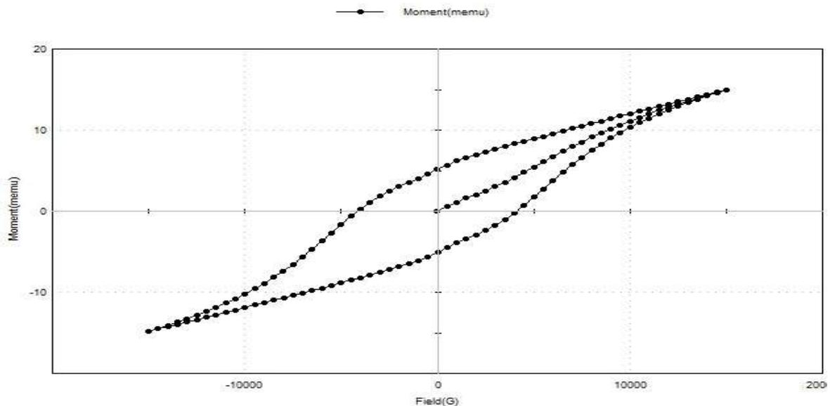
Fig 9 M-H Curve for as cast  $\alpha$ -Fe<sub>2</sub>O<sub>3</sub> powders annealed at 1000<sup>o</sup>C
