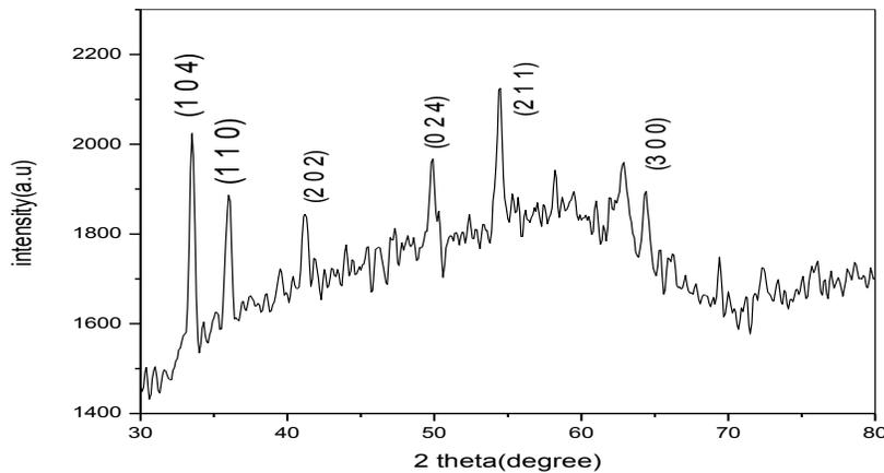
**Fig 5 X-ray Diffractogram of 15 hours milled and annealed  $\alpha$ -Fe<sub>2</sub>O<sub>3</sub> powders**
