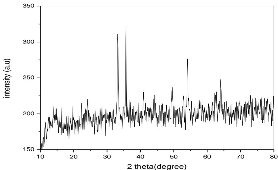
**Fig 1. X-Ray Diffractogram of  $\alpha$ -Fe<sub>2</sub>O<sub>3</sub> Powders**
