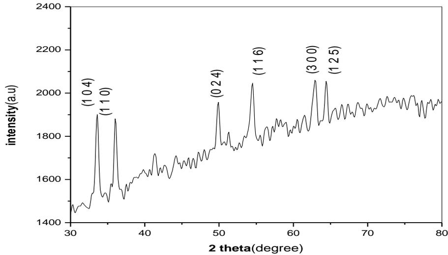
**Fig 4 X-Ray Diffractogram of  $\alpha$ -Fe<sub>2</sub>O<sub>3</sub> annealed powders**
