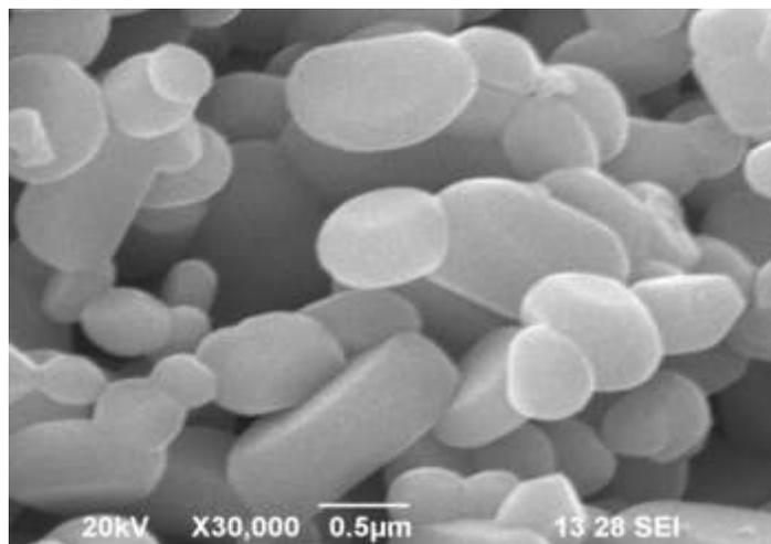
**Fig 7 SEM image of as cast  $\alpha$  -  $\text{Fe}_2\text{O}_3$  powder annealed at  $1000^\circ\text{C}$**
