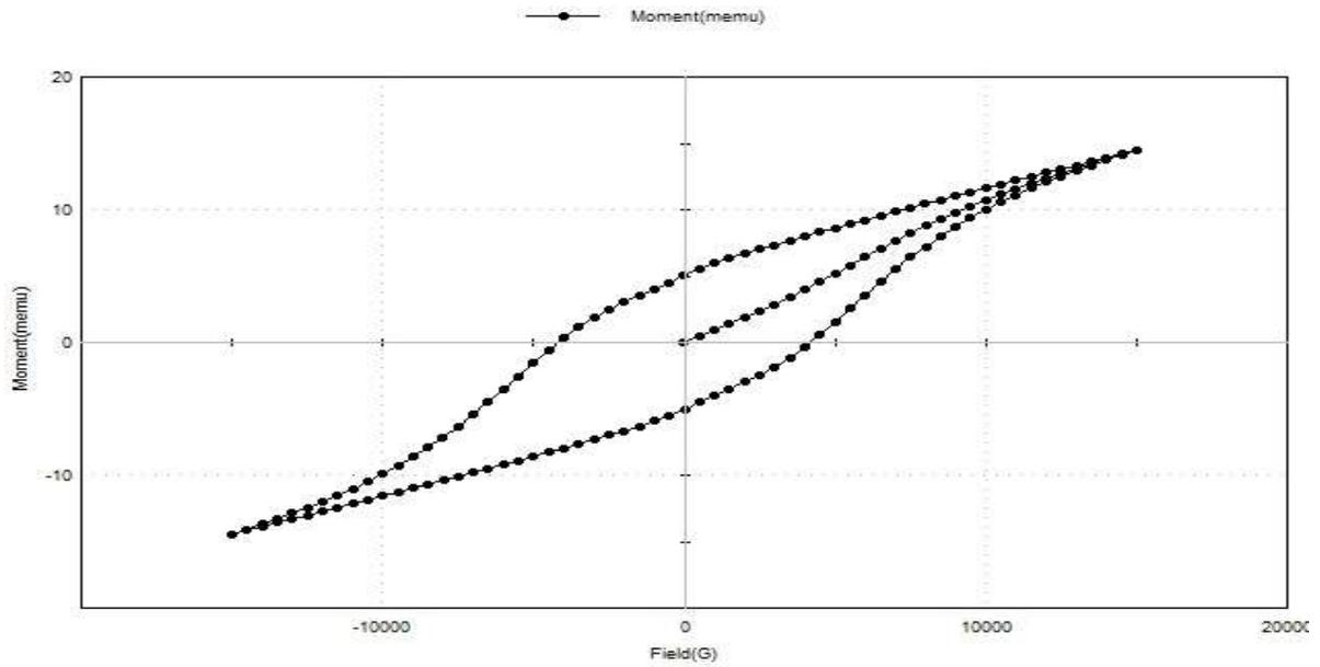
**Fig 10 M-H Curve for 25 hours milled  $\alpha$ -Fe<sub>2</sub>O<sub>3</sub> powders annealed at 1000<sup>o</sup>C**
