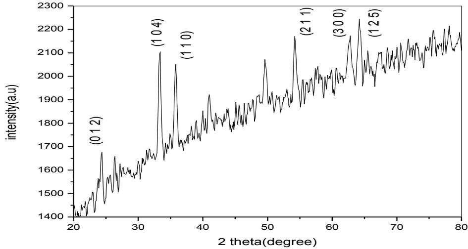
**Fig 6 X- Ray Diffractogram of 25 hours milled and annealed  $\alpha$ -Fe<sub>2</sub>O<sub>3</sub> powders**
