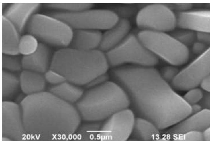
**Fig 8 SEM image of 25 hrs milled  $\alpha$ - $\text{Fe}_2\text{O}_3$  powders annealed at  $1000^\circ\text{C}$**
