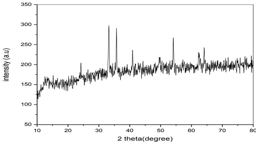
**Fig 3 X- Ray Diffractogram of 25 hours milled  $\alpha$ -Fe<sub>2</sub>O<sub>3</sub> Powders**
