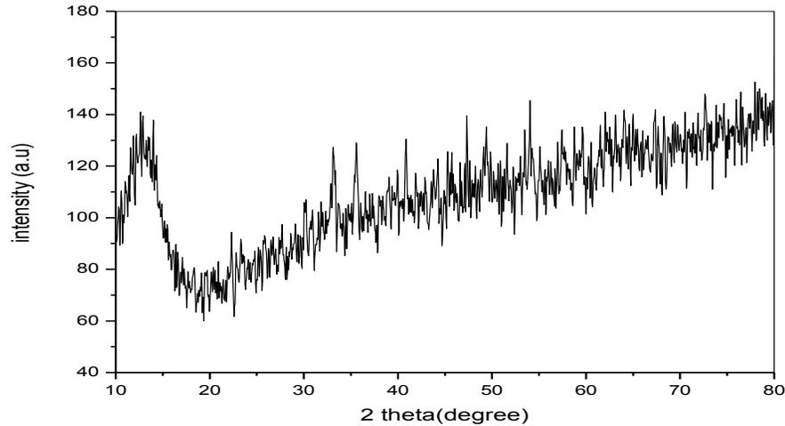
**Fig 2 X- Ray Diffractogram of 5 hours milled  $\alpha$ -Fe<sub>2</sub>O<sub>3</sub> Powders**
