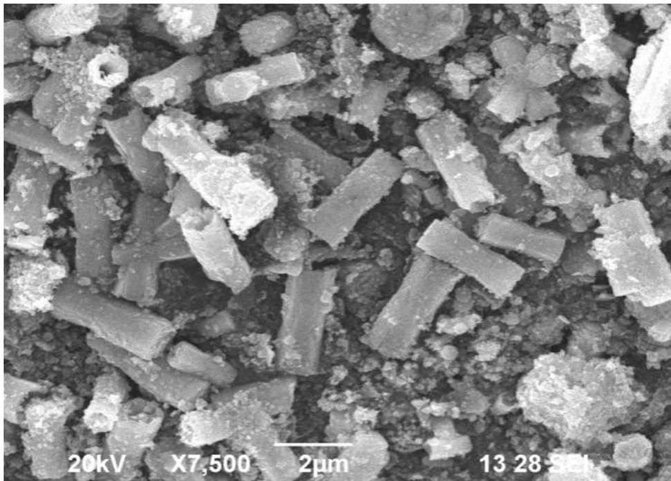
**Fig.5 SEM image of Ag doped ZnO**
