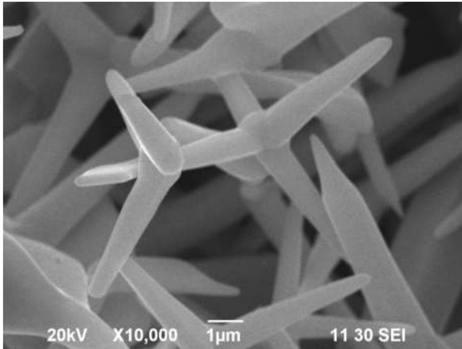
**Fig. 4 SEM image of undoped ZnO**
