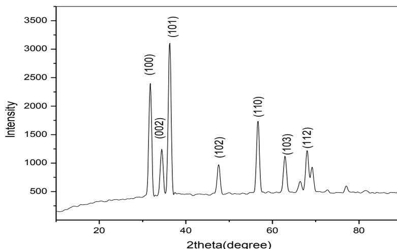
Fig. 1 XRD pattern of undoped ZnO nano particles
