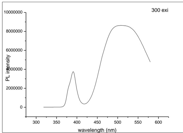
**Fig. 9 PL spectra of ZnO nano particles**
