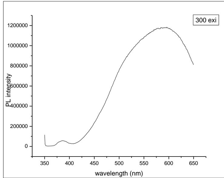
**Fig. 10 PL spectra of Ag doped ZnO nano structures**
