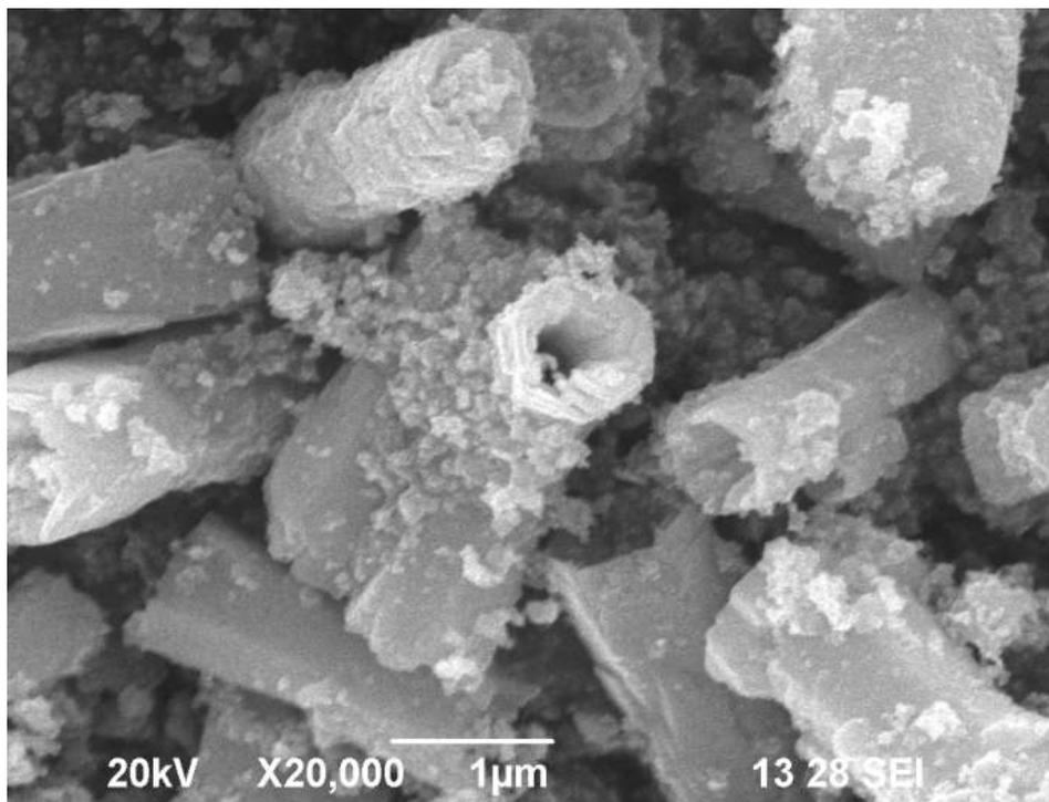
Fig 6: SEM image of Ag doped ZnO
