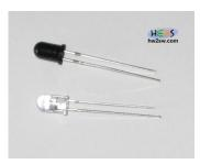
To detect car, Infrared TX/RX is used and simultaneously gives signal to PLC to trigger the respective compartment operation.
