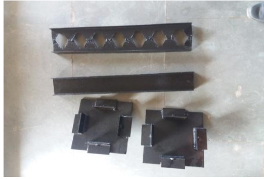
Photo 2 Fabricated section with end condition assembly
