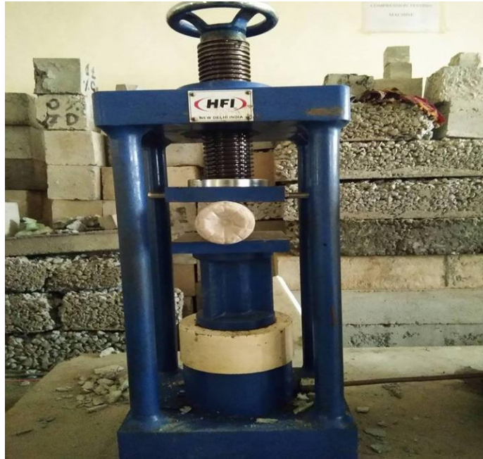
Fig. 3. Test applied on a waste PET bottles filled with soil and sealed tightly
