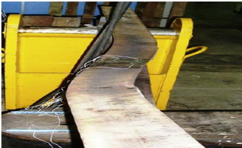
Fig 3 Lateral-Torsional Buckling of Castellated Beam
