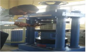
Photo no. 2 Rebound hammer test on cube
