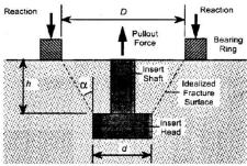
Fig 5 Pull out test
