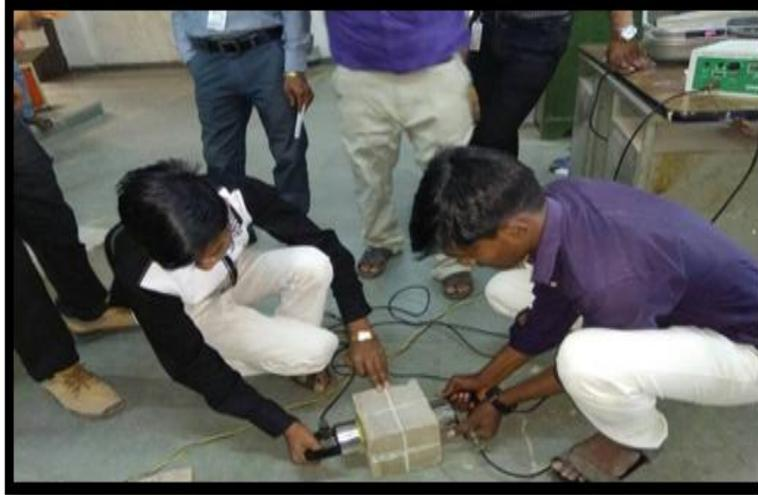
*Photo No.3 Ultrasonic Pulse Velocity
