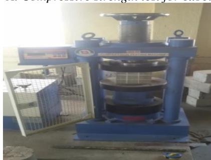
Photo No. 1 Compressive strength test for cube
