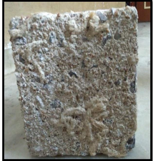
“Fig 2.6 Cube specimen after sulphate attack”
