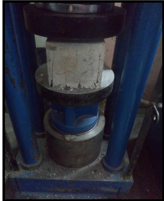
“Fig 2.2 Cube specimen after compression test”
