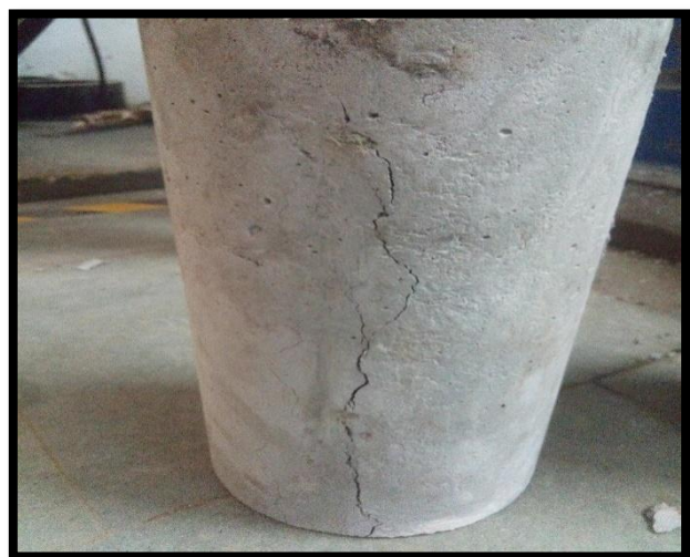
“ Fig 2.4 Cylindrical specimen after split tensile test”
