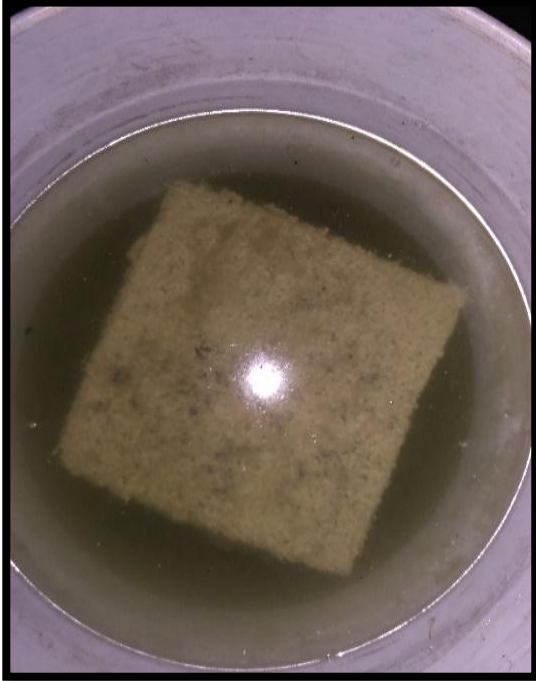
“Fig 2.5 Cube specimen immersed in H_2SO_4 solution”
