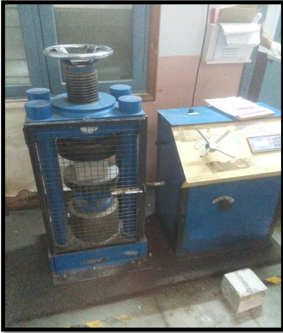
“Fig2.1 Compression Test on cube specimen”
