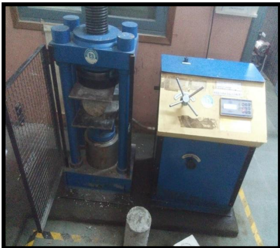
“Fig 2.3 Split Tensile Test on cylindrical specimen”
