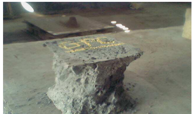
Fig.2-Failure Pattern of Cube After Testing
