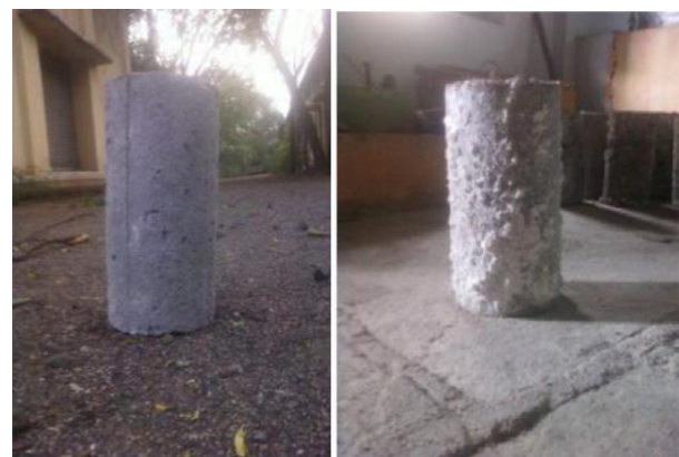
Fig.4-GPC and OPC specimens exposed to magnesium sulphate solution
