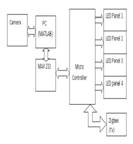
Fig 2.Block Diagram
