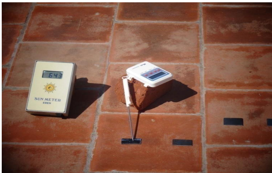
Figure 2. Measurement of temperature on absorber
