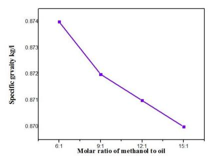
Figure 1. Effect of specific gravity with respect to molar ratio
