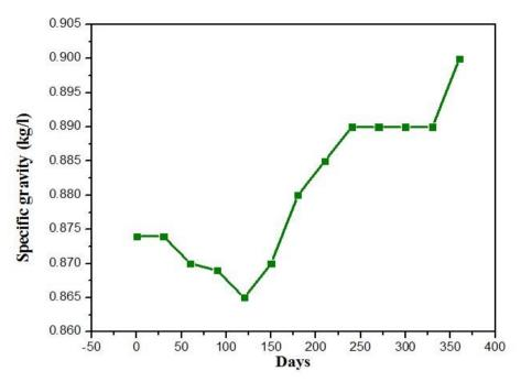
Figure 5. Chenges in specific gravity of biodiesel during storage
