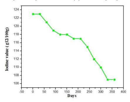
Figure 8. Changes in iodine value of biodiesel during storage.
