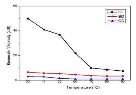
Figure 4. Comparison of kinematic viscosties of rubberseed oil, biodiesel and diesel inrelationship with temperature.
