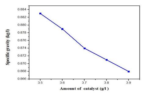
Figure 3. Effect of specific gravity with respect to catalyst.
