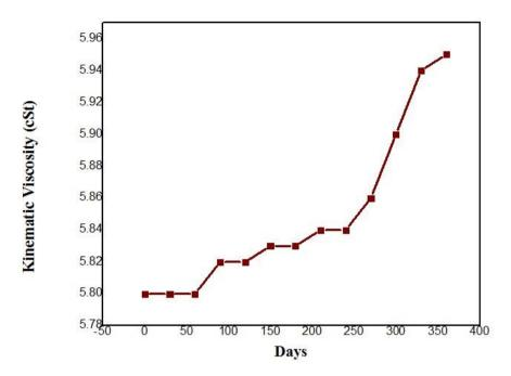
Figure 7. Changes in kinematic viscosity of biodiesel during storage.
