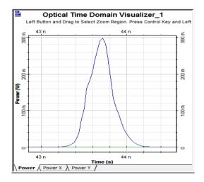
Figure 4.Simulation result for reduction of SPM effect after using MZM
