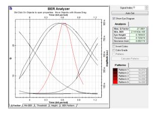
Figure 6.Eye diagram result for reduction of SPM effect
