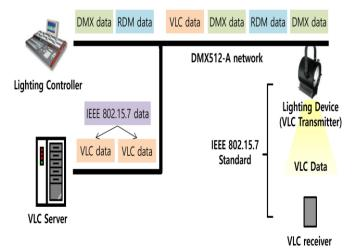
Fig.5 VLC Data Transmission on DMX512-A Network
