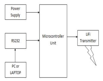
Fig.3 Block Diagram - Transmitter Unit
