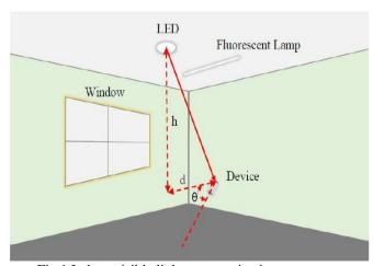
Fig.1 Indoor visible light communication system
