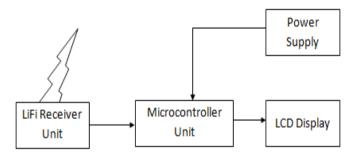
Fig.4 Block Diagram - Receiver Unit
