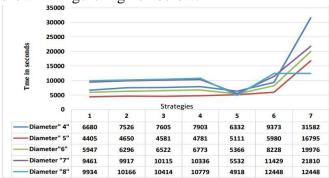
Figure 2.1: Relationship between Times spent in Machining to Different Strategies
